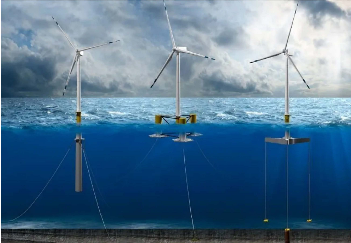
FIGURE 5-2 Common floating offshore wind support structures; (left to right) spar, semisubmersible, and tension-leg platform SOURCE: Cooperman et al., 2024. Illustration by Joshua Bauer, NREL.
