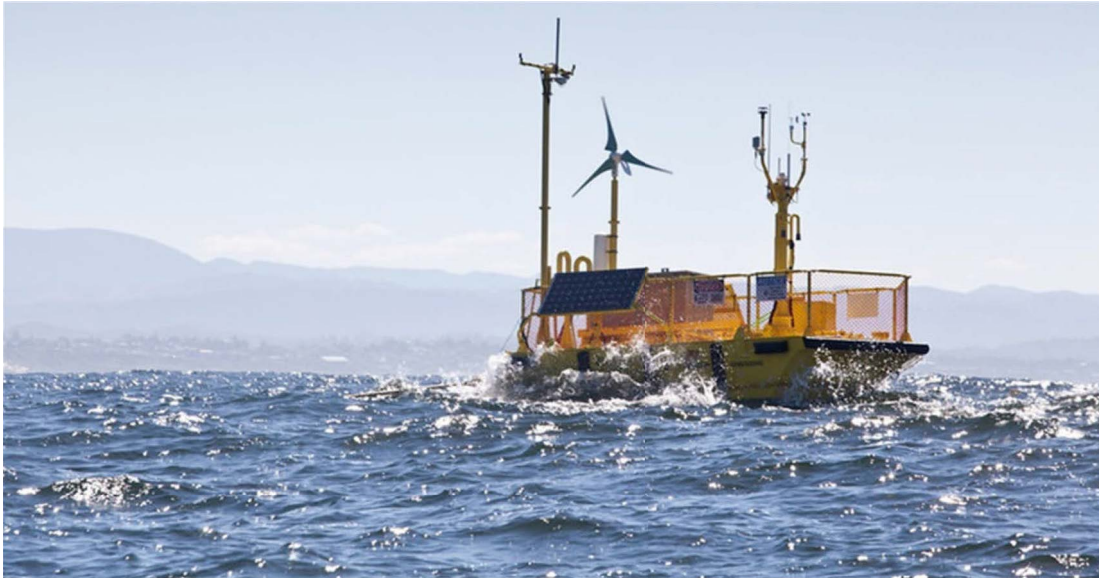
FIGURE 5-13 Ocean Sentinel mobile ocean test berth for non-grid-connected WECs at the PacWave North wave energy test site..
